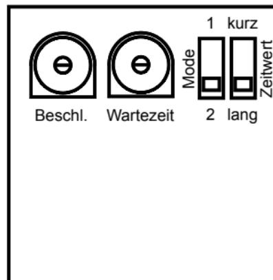
The time for a stop at a station is set by means of the „Pause“ switch and the „Wait Time“ setting controller on the circuit board.
